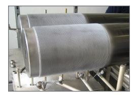
The PlasmaBond process is the application of a thin soft-metal film that, using a vacuum method, molecularly bonds the coating to the substrate. The two-part procedure results in superior bonding strength without affecting the properties of the underlying materials.
