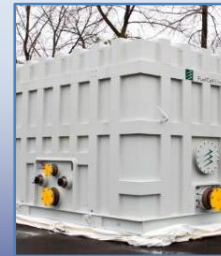
The stacks are enclosed, creating the fuel cell module
