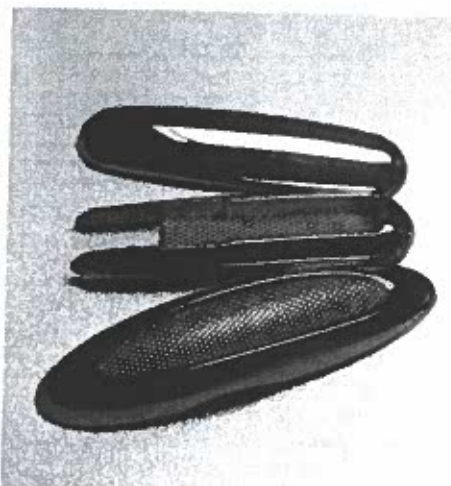
Fig. 9 Detail of textured MIM parts (Courtesy Gevorkyan)
