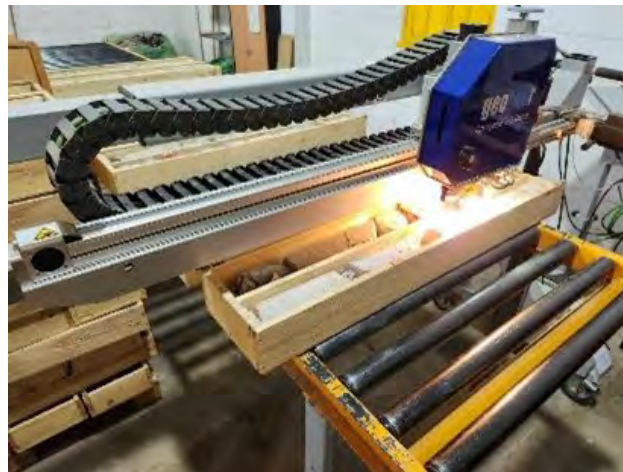
Figure 8.4: The geoLOGr hyperspectral scanning unit (McEwen 2023)
