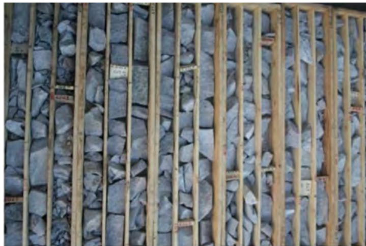
Figure 6.20: Typical drill core from Los Azules indicating the strongly fractured nature of the rock (Jemielita, 2010).
