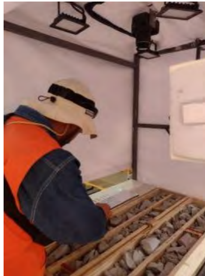
Figure 8.1: Dedicated static photo booth for consistent photography of core (McEwen 2023)
