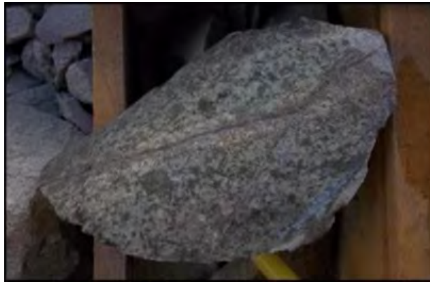
Figure 6.14: Typical drill core from Los Azules indicating the strongly fractured nature of the rock (Jemielita, 2010).
