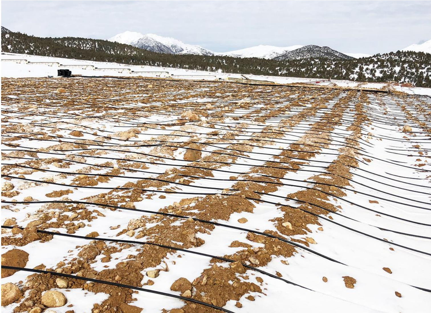
Solution Being Applied to Ore With Drip Tubing
