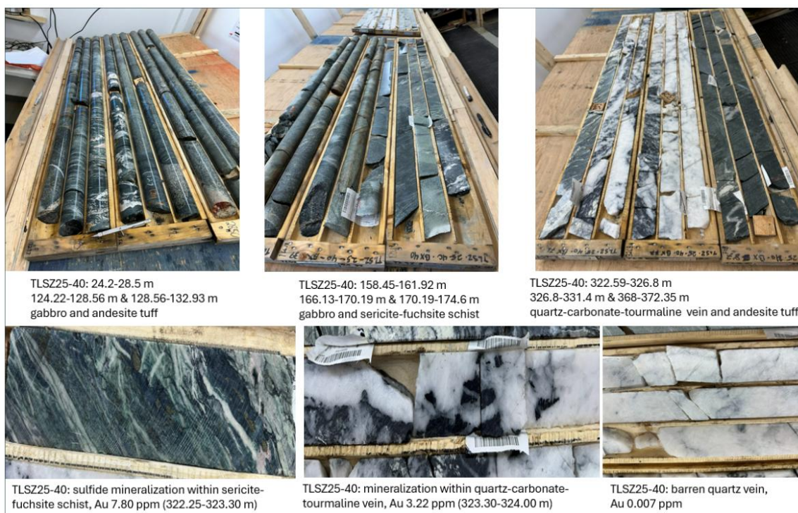
Photo 12-8: Visual Inspection of Selected Intervals from Hole TLSZ25-40
