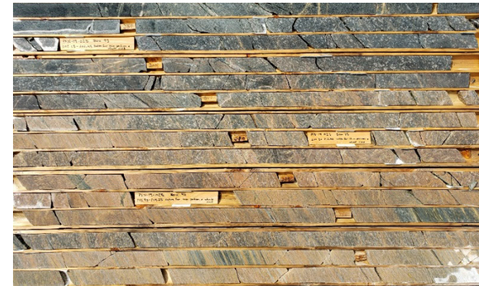
Progressively carb-silica-albite-musc-hematite altered and deformed porphyry
