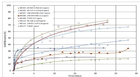
Figure 10: Leach kinetics of <30-day tests.
