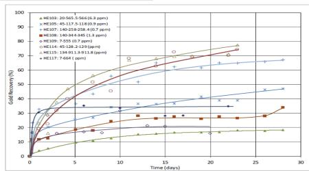
Figure 10: Leach kinetics of <30-day tests.
