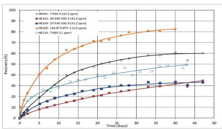
Figure 11: Leach kinetics of 30 to 50 day tests.
