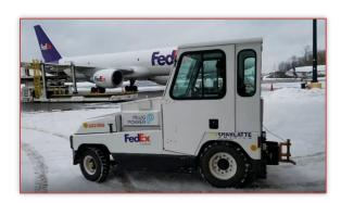
Plug Power deployed hydrogen-enabled ground support equipment at New York's Albany International Airport with FedEx. Powered by ProGen engines, the GSE vehicles transport packages from the airport sorting facility directly to FedEx airplanes while eliminating diesel emissions. Albany was selected to provide an excellent cold weather proving ground for the ProGen technology.
