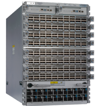
7800 R3 Up to 460Tbps 576 x 400G ports 36 x 400G, 48 x 100G LC Wirespeed, 2.5M Routes
