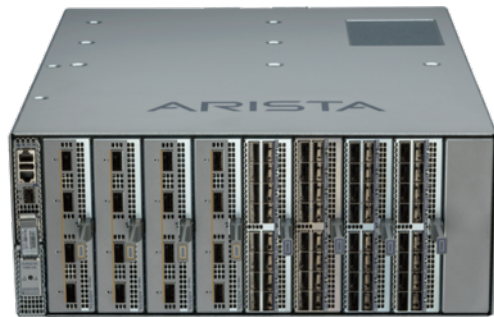
7368X4 Up to 128 x 100G 32 x 400G OSFP, QSFP-DD
