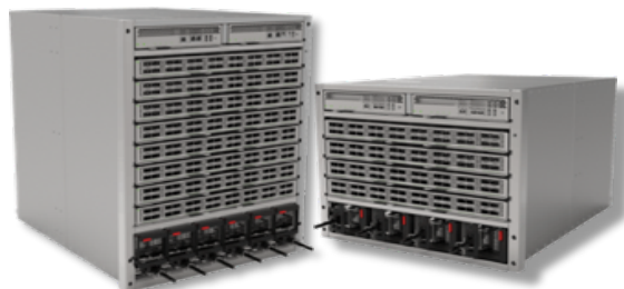
7300X3 4 & 8 Slot Modular System Up to 256 100G ports
